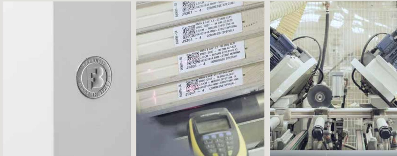
Highly automated machines allow us to obtain high precision during production and careful monitoring of all processes. An RFID tag is inserted into each door to ensure traceability and permit production data to be read automatically.
