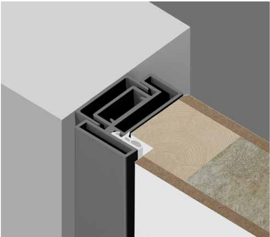
INNER C1 / flush on the push side
